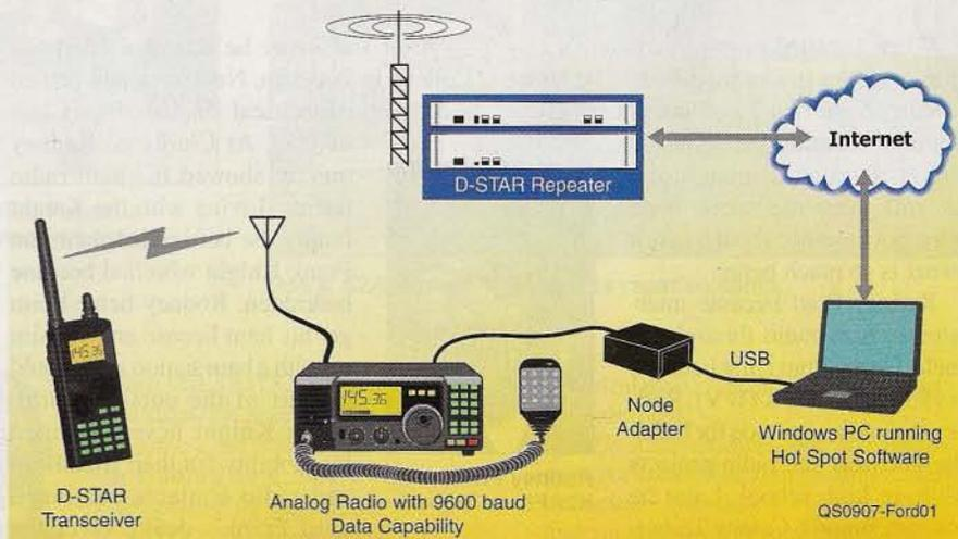
**Figure 1 — A D-STAR hot spot consists of an analog FM transceiver with 9600 baud data capability, a Windows PC running the hot spot software and an Internet connection. Thanks to the hot spot, the digital transmissions from your D-STAR radio will be received by the analog FM rig, decoded and passed to the D-STAR network via the Internet.**
